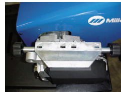
Independent drive roll pressure adjustment
